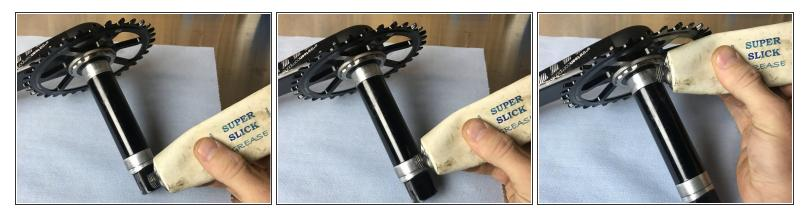
• With the BB already installed, start by greasing the crank spindle and polygon interface
