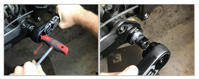
• Using the 8mm allen wrench turn counter-clockwise.
