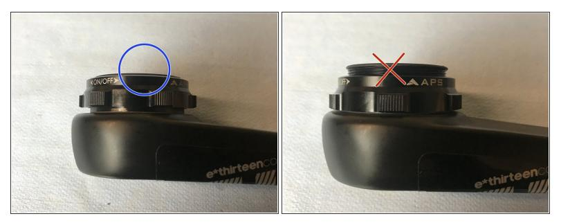
Before installing the arm turn the out ring of the APS adjuster such that the adjuster is in its flattest
