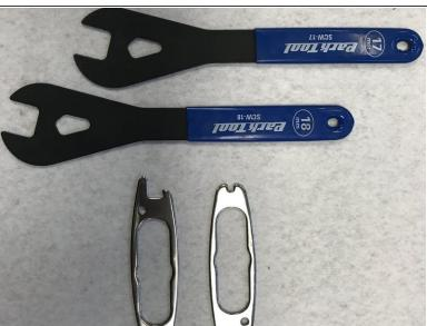
You will need a 17mm and 18mm cone wrench. \*\*The tools located in the bottom of the photo are included with aftermarket rear wheels.\*\*
