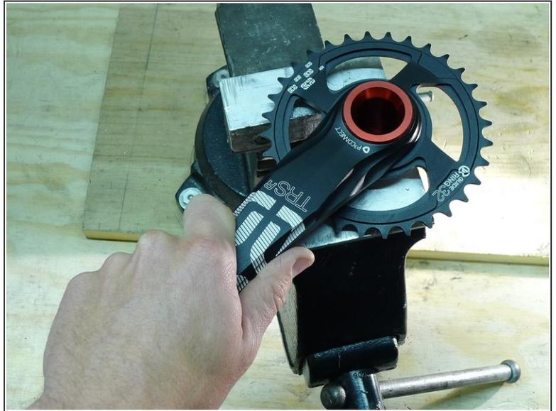
**⚠ Press down on the driveside arm and spindle assembly to ensure that it does not slip in the tool**
