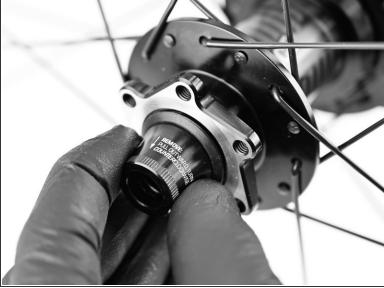
• Install non-drive axle endcap. Apply pressure and tighten clockwise until endcap spins freely.
