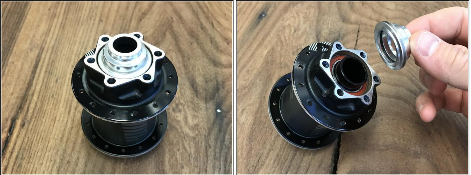
**⚠ Any brand bearing press will work as long as the correct size bearing drifts are used. DO NOT HAMMER OUT BEARINGS - This can lead to a debonded hub shell.**
