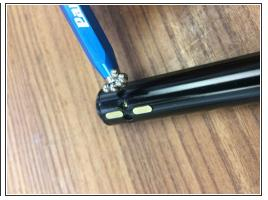
With pillar removed from the inner tube, use a magnet to keep the balls from disappearing
