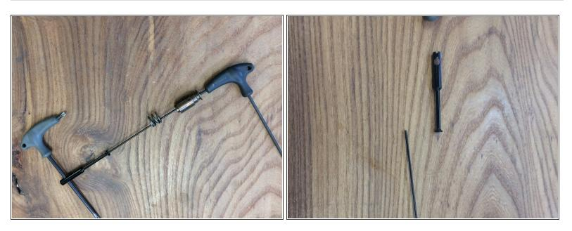
Use an M3 hex wrench and any tool that will fit into the cable slot to un-thread the cable holder from the spoke
