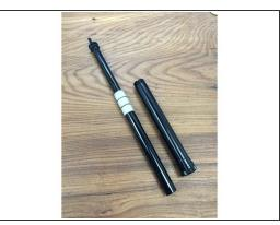
Slide the outer tube up to remove it from the post
