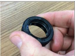
Remove the main seal from the outer tube by turning it counter-clockwise
