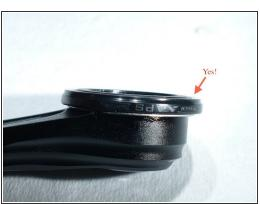
Before installing the arm turn the out ring of the APS adjuster such that the adjuster is in its flattest position
